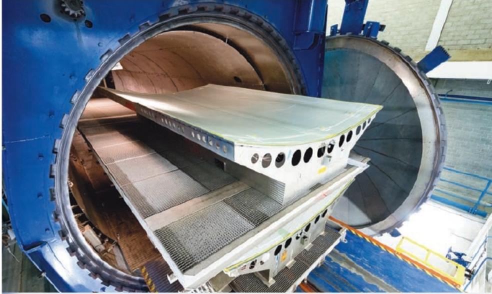
Figure 1.10: Large autoclave for curing completely assembled A380 Glare panels[17]
