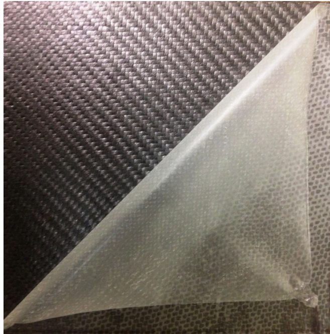
Figure 3.3: Woven carbon fiber/epoxy prepreg before curing.
