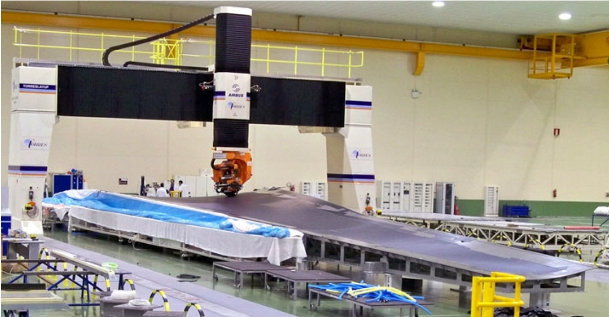
Figure 1.9: Automated tape layer machine [16]
