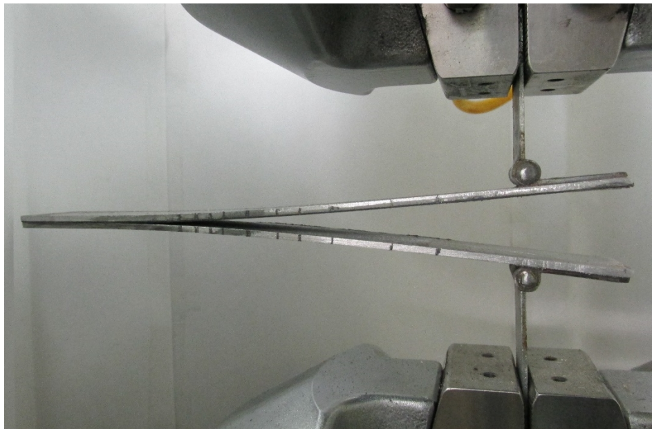
Figure 3.12: T-Peel test being conducted.
