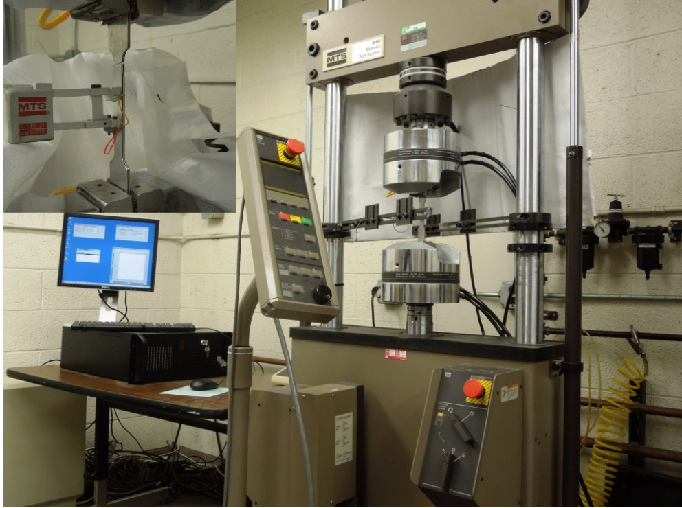
Figure 5.2: Tensile test setup with MTS machine.
