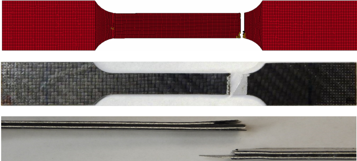
Figure 5.17: FEA and experimental failed specimen of CARALL-B having veil cloth layers
