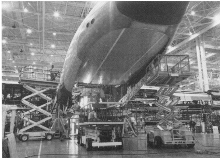
Figure 1.11: First ARALL cargo door installed on the C-17, February 27, 1991.[21]
